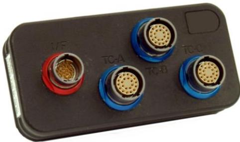
The TIU-32 is a 32 channel thermocouple interface unit. Two versions are available, the TIU-32 and the TIU-32C providing output as either 0-5V analogue or via CAN.
